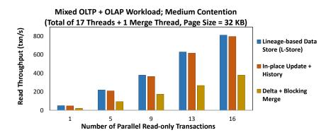
Coping with tens of update threads with a single merge thread
