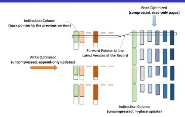
Achieving (at most) 2-hop access to the latest version of any record (avoiding read performance deterioration for point queries)
