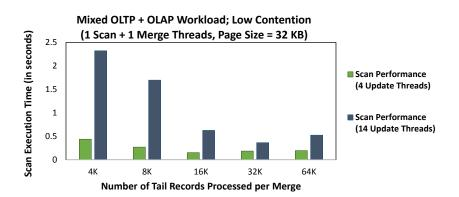
Merge process is essential in maintaining efficient scan performance
